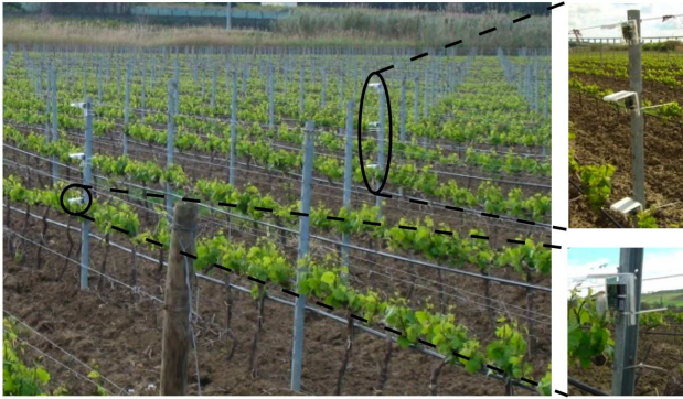
Figure 2. The WSN deployment in the vineyard.
