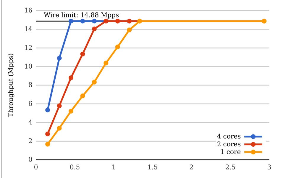
**netmap** uses 70..90 CPU clocks to send or receive one packet, 10-20 times less than standard APIs, and has with very good scalability on clock frequency and number of cores.
